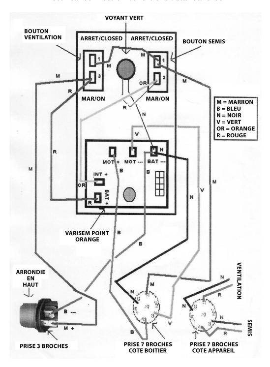
Switch  $n^{\circ}1$  is used to start the tray. Switch  $n^{\circ}2$  is used to start the endless screw
