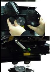
3. Unscrew the 2 knurled knobs holding the grease bearing
