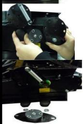
3. Unscrew the 2 knurled knobs holding the grease bearing
