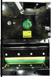
The two knurled buttons, the rotor grease bearing and its 2 washers
