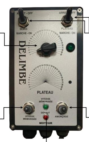
2. Installing your GPS antenna outside the cab and switch on your machine, sowing and plate ON and start seeding.
