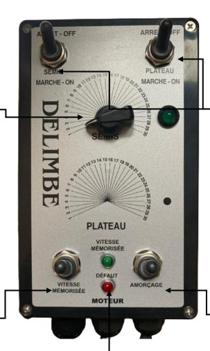
2. Install your sensor on a rotating element and switch on your machine, sowing and plate ON and start seeding.
